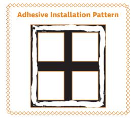
Set an XL Block on the initial starting line. Use the Wakol MS 245 Caulk adhesive to apply a 1/4" bead of caulk along the outside perimeter of the XL Block - do not apply adhesive to the interior connector pieces (see above image).
