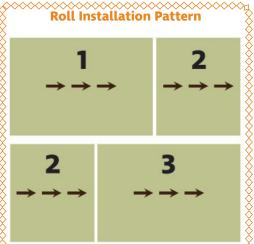
as possible. **Failure to follow correct roll sequencing could cause excessive shade variation or gapping at seams.** Head seams must be staggered by 6' – 10' (depending on room size and roll length) and must be cut prior to installing material with adhesive. When installing out of sequence, cutting multiple pieces from one roll, cutting head seams or side seams, the material must be overlapped and double cut or trace cut to provide a more seamless appearance.
