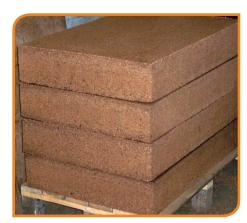
blocks are baked at varying temperatures to produce the different shades of color seen within the Mediterra line - the darker the color, the higher the temperature and the longer the baking time. Once baked, the blocks are cut into tiles and planks.
