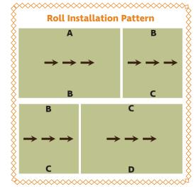
Ensure seams have a consistent visual appearance at edges so that color variations blend as seamlessly as possible. Overlap seams by ~1/16" to ensure tight seams during final installation. Horizontal seams must be staggered by 6' – 10' (depending on room size and roll length) and must be cut prior to installing material with adhesive. Ensure flooring seams do not directly overlap seams in substrate.
