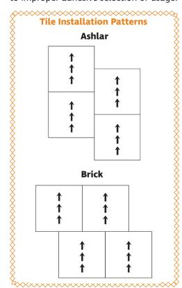
Prior to installation, confirm material installation pattern and direction per design specifications or work order. Manhattan tile should be installed in an ashlar or brick pattern to ensure tight seams and an overall ideal visual appearance. Ensure that directional
