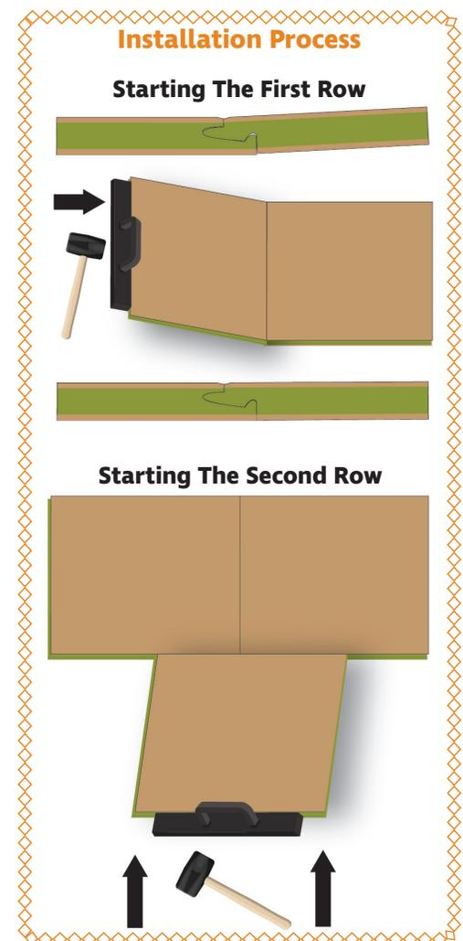
Once the installation has reached the center line, finish installing the row along the center line and shift or adjust entire installed flooring section as necessary. If perimeter planks need to be installed after adjusting installation, install perimeter planks before continuing with installation, ensuring perimeter gaps are installed per section 5. Ensure all perimeter planks are at least 10" in length and 6" in width to avoid installation issues.
