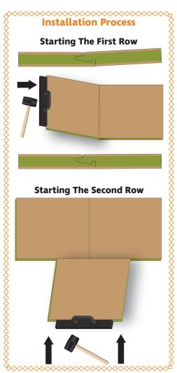
Once the installation has reached the center line, finish installing the row along the center line and shift or adjust entire installed flooring section as necessary. If perimeter planks need to be installed after adjusting installation, install perimeter planks before continuing with installation, ensuring perimeter gaps are installed per section 5. Ensure all perimeter planks are at least 10" in length and 6" in width to avoid installation issues.
